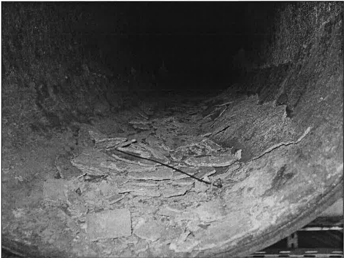
Fig. 4: Photo of LSA scale at the bottom of the oil export pipe on the Papa side.
